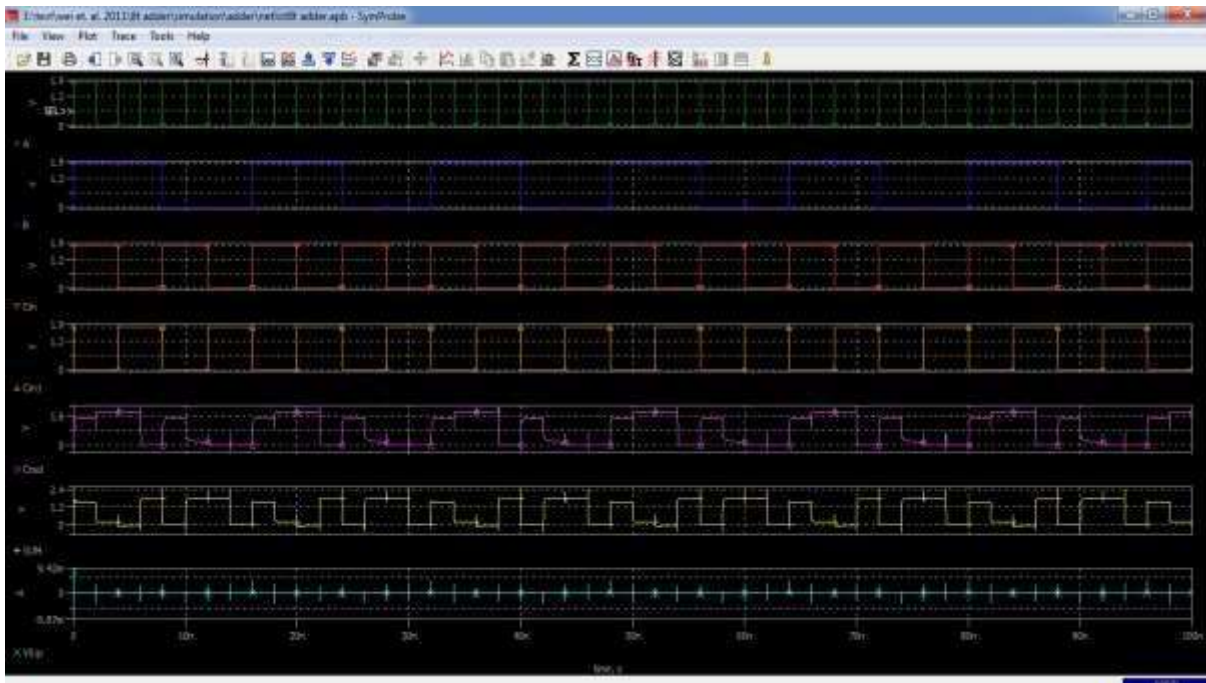
Fig. 9. Output waveforms of wei et. al. 2011 8-T adder in Symprobe software
